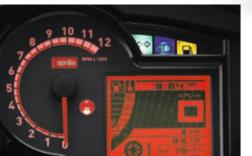
WE SHOULD CERTAINLY NOT OVERLOOK THE BRAND NEW **ACTIVE MATRIX DIGITAL DASHBOARD** WITH ANALOG REV COUNTER AND GENEROUS LCD DISPLAY FOR FUEL, COOLANT TEMPERATURE, CLOCK, SPEEDOMETER, MILEOMETER AND TWO TRIP COUNTERS, JOURNEY TIME AND MAXIMUM SPEED, 16 MEMORY TIMER, BATTERY VOLTAGE, AND COMPLETE DIAGNOSTICS. YOU CAN EVEN ACCESS ALL THESE FUNCTIONS DIRECTLY FROM A CONTROL ON THE HANDLEBARS.
